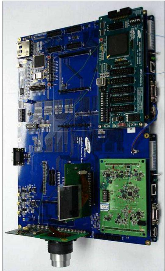
Figure 1: Initial Samsung FPGA DSC Platform using S5C7380x
