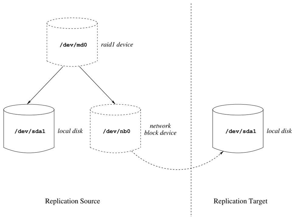
Figure 1: Data replication using raid1 over nbd
