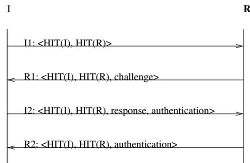
Figure 2: The base exchange of the Host Layer Protocol
