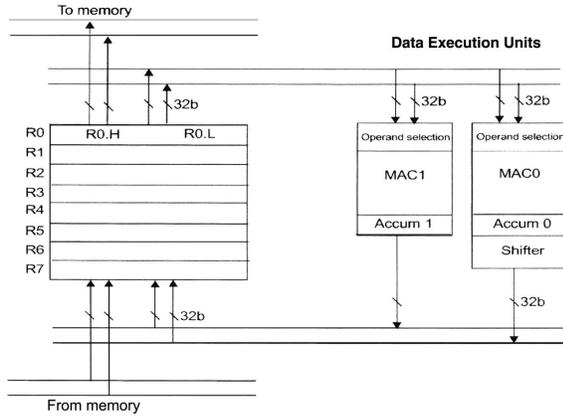
Figure 3: Register Files and Execution Unit
