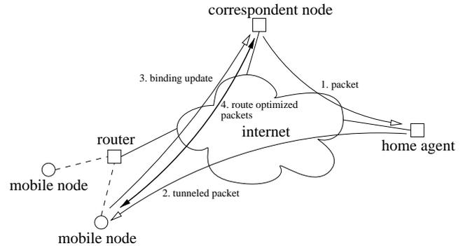
Figure 1: Mobile IPv6 Operation
